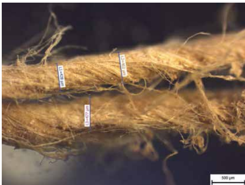
Fig. 3. Thickness measurement on the yarn used for jar IF 1910, observed in reflected light, magnification 4x; slightly Z twisted fibers, diameter 0.5 – 0.6 mm.
