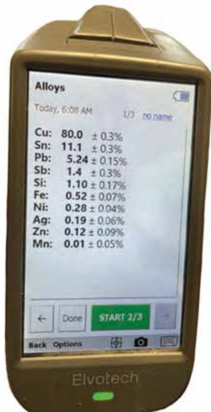
Fig. 6. Performing pXRF measurements on the three-legged metal container with wooden handle (IF 1590) and the result on the display of the device.
