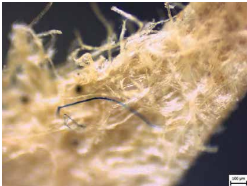
Fig. 2. Paper sample taken from jar IF 1905, observed in reflected light, magnification 4x.
