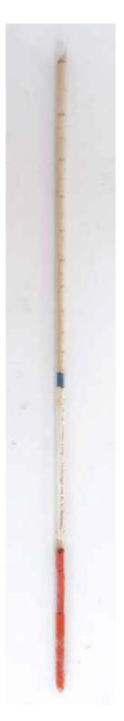
New inventory no.: IF 1894. Type: aerometer. Dating: 19<sup>th</sup> – early 20<sup>th</sup> century. Dimensions: preserved length: 48 cm, diameter: 0.5 cm. Materials: paper, glass, red wax? Description: Glass density meter, with both printed text, in German, and handwritten grading inside. The end
