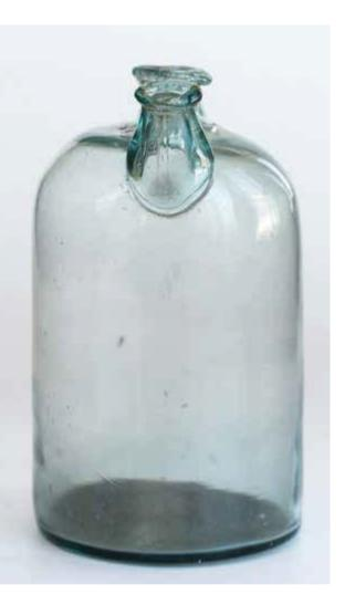
New inventory no.: IF 319. *Type*: laboratory glassware. Dating: mid-19<sup>th</sup> century. Dimensions: no measurements on record. *Materials*: clear blueish glass. Content: not preserved. Description: Wulf jar made of transparent blueish glass, with three necks. *Context of use*: the Crown of Hungary pharmacy in Baia Mare. *State of preservation*: good. Date of acquisition: 1963. Observations: pontil mark on the bottom, free-formed, air bubbles in the paste, irregular necks and rims.
