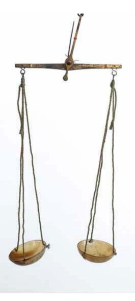
New inventory no.: IF 2374. Type: apothecary scale. Dating: early 20<sup>th</sup> century. Dimensions (old measurements): height: 26 cm, beam length: 10.1 cm, pans diameter: 2 cm.
