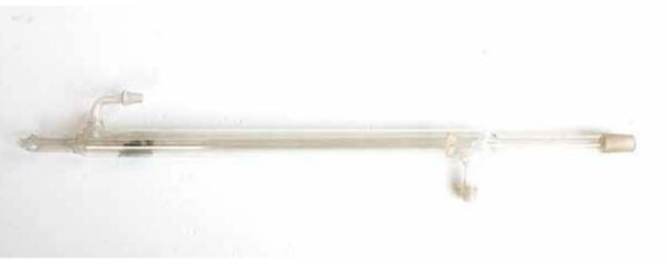
New inventory no.: IF 592. Type: laboratory glassware. Dating: 19<sup>th</sup>-20<sup>th</sup> century. Dimensions: length: 48 cm, openings diameter: 3.5 / 2.4 cm. Materials: clear glass. Description: Distillation tube with two openings, one larger, stained. Context of use: the Pomegranate pharmacy in Oradea. State of preservation: good, accretions, chippings in the rim. Date of acquisition: 1963.
