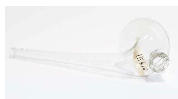
New inventory no.: IF 616. Type: laboratory glassware. Dating:  $19^{th}-20^{th}$  century. Dimensions: length: 21 cm, short neck diameter (inner): 1.3 cm, tube diameter (inner): 0.6 cm. Materials: clear glass. Description: Retort flask, made of clear glass, upper opening with applied collar. Context of use: the Hintz pharmacy in Cluj-Napoca. State of preservation: good. Date of acquisition: 1963.
