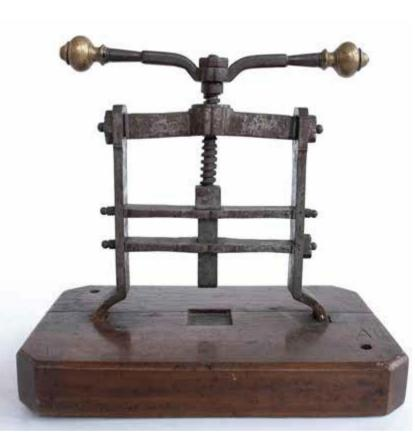
New inventory no.: IF 1611. *Type*: press. Dating: 19th century. Dimensions: no measurements on record. Materials: metal. Description: Large seal press, frame made of forged iron bar bolted together with nuts. Central vertical threaded rod, handle bar with spherical brass finials. Lower end of the ram fitted with receiver for signets (missing the retaining screw). Mounted on solid wooden stand.
