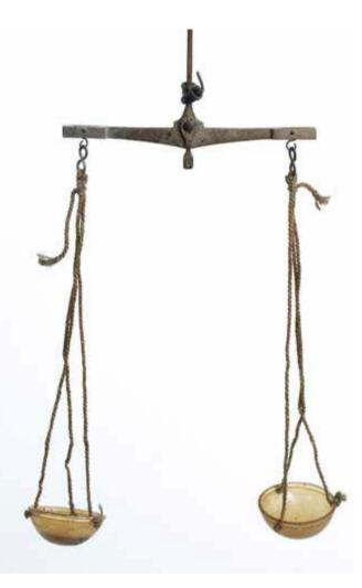
New inventory no.: IF 2376. *Type*: apothecary scale. *Dating*: early 20<sup>th</sup> century. Dimensions (old measurements): height: 26 cm, beam length: 10.1 cm, pans diameter: 2 cm. *Materials*: metal, string, plastic. Description: Apothecary scale (equal arm balance) with two ebonite bowl pans, small and very concave, each hanging by three brown textile strings, with needle pointer and hook in the upper part. Needle secured in place with wire for display purposes.
