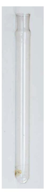
New inventory no.: IF 1896. Type: test tube. Dating: 19<sup>th</sup> – early 20<sup>th</sup> century. Dimensions: no measurements on record. Materials: clear glass. Description: Clear glass text tube with difference in diameter toward the mouth. Used with density meters. Context of use: the Hintz pharmacy in Cluj-Napoca. Date of acquisition: 1963. State of preservation: good.
