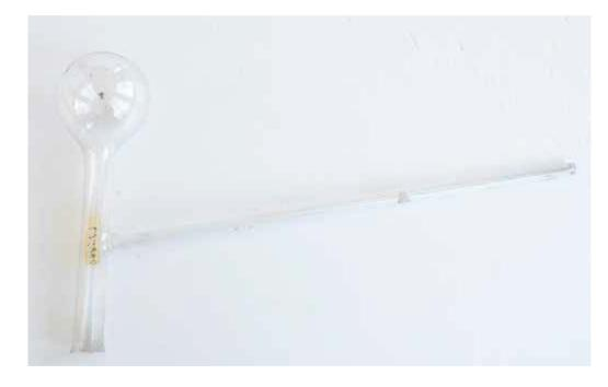
New inventory no.: IF 1881. Type: laboratory glassware. Dating: early 20<sup>th</sup> century. Dimensions: side tube length: 19.5 cm, flask tube length: 8.5 cm, tube diameter: 0.4 cm, neck diameter: 1.2 cm. Materials: clear glass. Description: Two glass tubes meeting at an angle, one ending in a widened, broken part, likely from a flask (similar to cat. 383). Context of use: the Hintz pharmacy in Cluj-Napoca. State of preservation: bad, missing piece.
