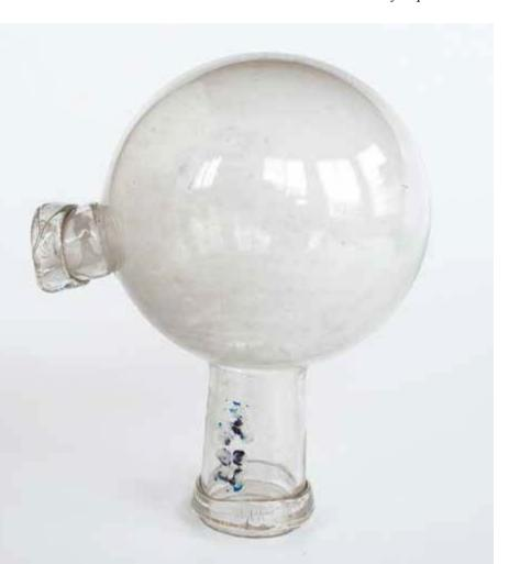
New inventory no.: IF 601. *Type*: laboratory glassware. Dating: 19<sup>th</sup>–20<sup>th</sup> century. Dimensions (old measurements): tube height: 17.7 cm, flask height: 13 cm, flask maximum diameter: 6.5 cm. Materials: clear glass. Description: Florence flask made of clear glass, with long tube sideways, from the neck, and then downwards. Context of use: the Hintz pharmacy in Cluj-Napoca.
