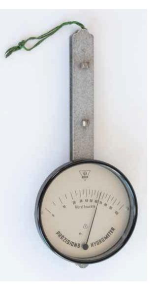
New inventory no.: IF 2053. Type: hygrometer. Dating: 20<sup>th</sup> century. Dimensions: height: 28 cm, diameter: 12 cm, thermometer length: 11.5 cm.
