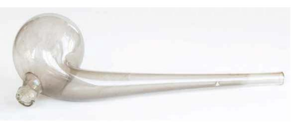
New inventory no.: IF 612. Type: laboratory glassware. Dating:  $19^{th}-20^{th}$  century. Dimensions (old measurements): length: 56 cm, maximum width: 27 cm, opening diameter: 2.8 cm. Materials: clear glass. Description: Retort flask, made of clear glass, upper opening with applied collar. Context of use: the Hintz pharmacy in Cluj-Napoca. State of preservation: good, accretions. Date of acquisition: 1963.
