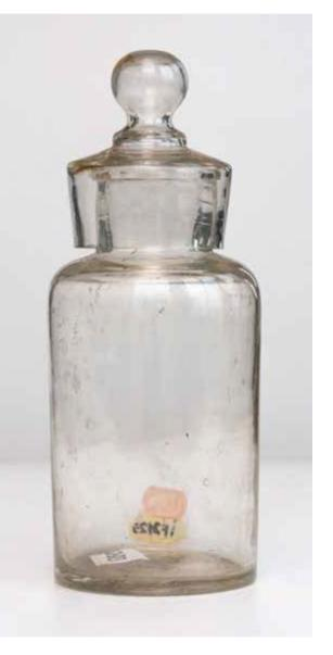
New inventory no.: IF 2123. No. of items: 2. Type: glass container. Dating: 19<sup>th</sup>-20<sup>th</sup> century. Dimensions (old measurements): height: 21.3 cm, base diameter: 10.2 cm, mouth diameter: 6.5 cm. Materials: clear glass. Content: not preserved. Description: Clear glass laboratory container with loose glass bell-like cover with cupping cup-shaped knob. Capacity embossed on the base.
