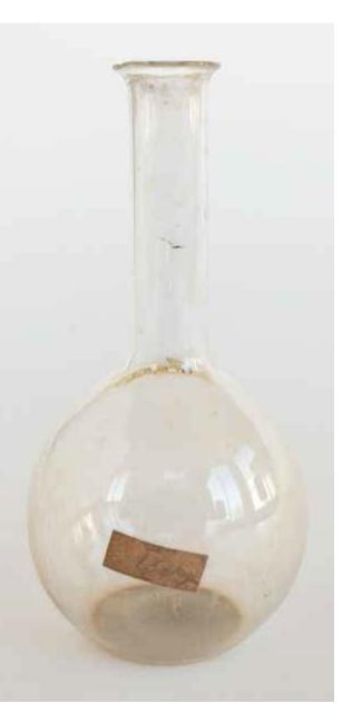
New inventory no.: IF 602. Type: laboratory glassware. Dating: 19<sup>th</sup>-20<sup>th</sup> century. Dimensions (old measurements): height: 17 cm, base diameter: 4.8 cm, mouth diameter: 2.8 cm. Materials: clear glass. Description: Volumetric flask made of clear glass. Context of use: the Hintz pharmacy in Cluj-Napoca. State of preservation: good, browned paper label, accretions. Date of acquisition: 1963.
