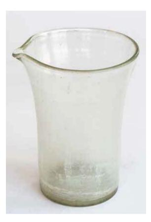
New inventory no.: IF 2410. Old inventory no.: ? Type: laboratory glass. Dating: mid-19<sup>th</sup> century. Dimensions: no measurements on record. Materials: clear glass. Content: not preserved. Description: Clear glass laboratory container, with tall curved spout and circular short tube on one side of the neck. State of preservation: good, accretions.
