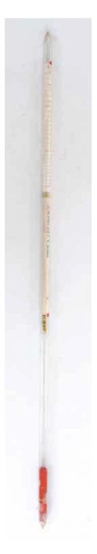
New inventory no.: IF 1890. Type: aerometer. Dating: 19<sup>th</sup> – early 20<sup>th</sup> century. Dimensions: length: 50 cm, diameter: 0.5 cm. Materials: paper, glass, red wax? Description: Glass density meter, with both printed text, in German, and handwritten grading inside. Inscription: on paper inside the tube: F.X. Kukla nach P. T. Meissner... Context of use: the Hintz pharmacy in Cluj-Napoca. Date of acquisition: 1963. State of preservation: good.
