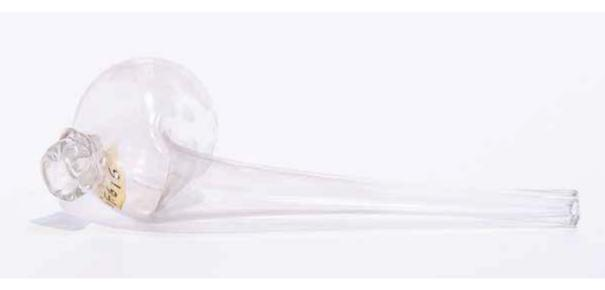
New inventory no.: IF 617. Type: laboratory glassware. Dating: 19<sup>th</sup>-20<sup>th</sup> century. Dimensions (old measurements): length: 24.5 cm, maximum width: 8 cm, opening diameter: 1.5 cm. Materials: clear glass. Description: Retort flask, made of clear glass, no upper opening. Context of use: the Hintz pharmacy in Cluj-Napoca. State of preservation: good. Date of acquisition: 1963.
