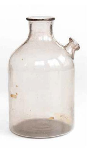
New inventory no.: IF 1786. *Type*: laboratory glassware. Dating: mid-19<sup>th</sup> century. Dimensions (old measurements): height: 21 cm, base diameter: 12.4 cm, large-mouth diameter: 5.2 cm, smallmouth diameter: 2.7 cm. Materials: clear glass. Description: Wulf jar made of transparent glass, with two necks and mouths - a larger one, in the center, and a smaller one, on the side. *Context of use*: the Unicorn pharmacy in Cluj-Napoca. State of preservation: good, accretions.
