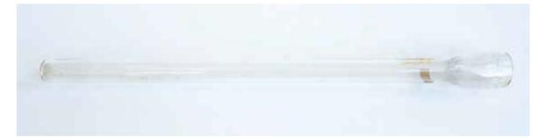
New inventory no.: IF 608. Type: laboratory glassware. Dating: 19<sup>th</sup>-20<sup>th</sup> century. Dimensions: length: 48 cm, openings diameter: 3.5 / 2.4 cm. Materials: clear glass. Description: Distillation tube with two openings and broken side tube. Made of clear glass. Context of use: the Hintz pharmacy in Cluj-Napoca. State of preservation: bad, broken end.
