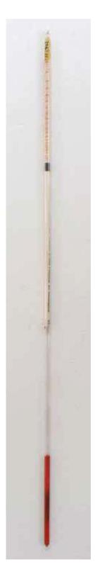
New inventory no.: IF 1902. Type: alcoholmeter. Dating: 19<sup>th</sup> – early 20<sup>th</sup> century. Dimensions: length: 54 cm, diameter: 0.4 cm. Materials: paper, glass, red wax?
