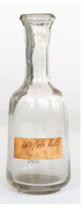
New inventory no.: IF 1042. Type: measuring bottle. Dating: 1910. Dimensions (old measurements): height: 21 cm, base diameter: 7.7 cm, mouth diameter: 4.5 cm. Materials: clear glass, paper. Description: Measuring bottle made of transparent glass, with tall, slightly flaring neck. Handwritten notations in black and blue ink on a rectangular paper label, notations incised below the rim. Half liter capacity. Inscription: on the label: 667/910 kih
