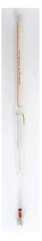
New inventory no.: IF 1889. *Type*: aerometer. *Dating*: 19<sup>th</sup> century. Dimensions: length: 34 cm, maximum width: 2 cm. *Materials*: paper, glass, mercury. Description: Glass density meter with mercury, with handwritten inscription inside (in German) on paper label and grading with black and white numbers. *Inscription*: on paper inside the tube: Leichtmeszer bei +15° Reaumur, on the glass: 5 cm? Context of use: Sibiu. *State of preservation*: good. Date of acquisition: 1963.
